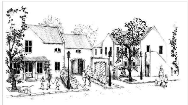
Figure 4: Illustration of typical street elevation illustrating edge continuity with pedestrian "poort" used as linking element.
